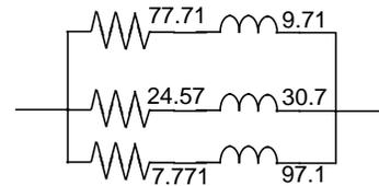
**Fig.2: 3 Branch Ladder in  $m\Omega$  and  $nH$**
