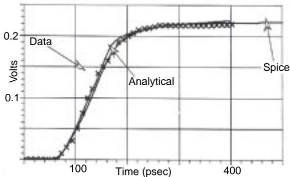
Fig.4: Comparison of the Data, Spice simulation and Analytical results are shown here. The sample is a 5 meter co-axial cable. The Y axis is Voltage and the X axis is time in seconds.
