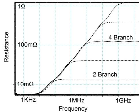
**Fig.3a & 3b: Inductance & Resistance plot for 1-6 ladder circuits**
